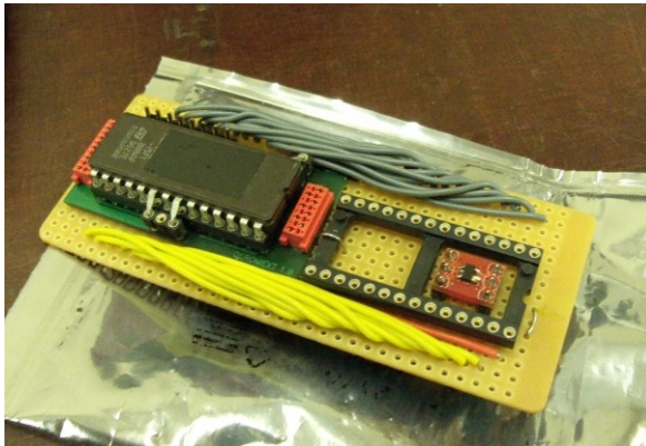
Picture of a prototype QL ROMExt board (picture courtesy of Memory Lane Computing)
